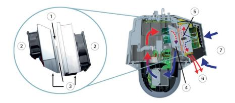
Peltier element (1) draws heat out of or into the camera as needed; forms part of the barrier separating the camera unit from the outer environment. (2) Fan. (3) Heat sinks. (4) Air-tight camera compartment; no air flow between camera unit and outer part. (5) Heat inside is transferred out. (6) Warmer air out (7) Cooler air in.
